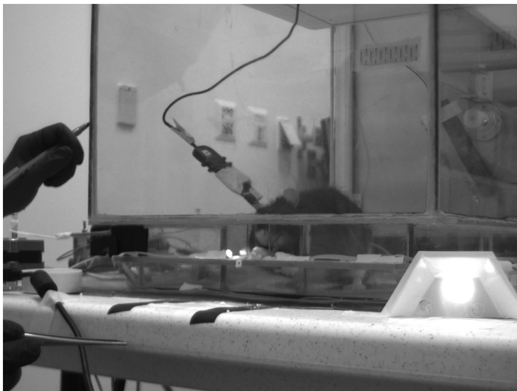
Image 4. Example frame from 2 nd video camera depicting a side view. LED indicators in view at bottom right, with the middle LED signifying an infrared beam break has occurred.
