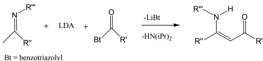
Scheme 2.1 – Synthesis of ketoimines by reaction of acylbenzotriazoles.
