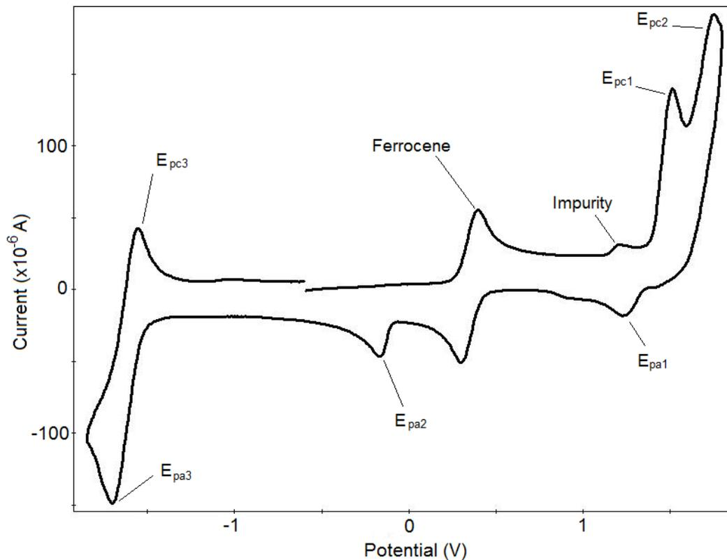
Figure 3.11 – CV of 4.65 mM 5b in CH<sub>2</sub>Cl<sub>2</sub> on a GC electrode at 24.5 °C, 0.7 M [tBu<sub>4</sub>N][PF<sub>6</sub>],  $\nu = 0.2 \text{ V s}^{-1}$  referenced to ferrocene.
