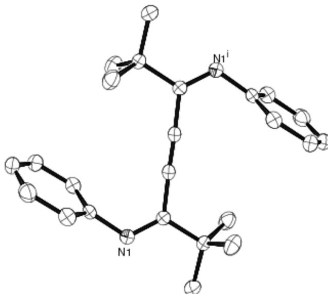
Figure 3.8 – ORTEP diagram for alkynyl diimine **5a**. Hydrogen atoms omitted for clarity (50% probability ellipsoids shown). Ni<sup>i</sup> was generated by a centre of symmetry.
