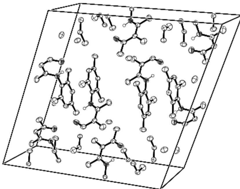
Figure 2.6 – ORTEP diagram of the unit cell contents of 1d showing the  $\pi$ - $\pi$  stacking of the mesityl substituents. Hydrogens are omitted for clarity.
