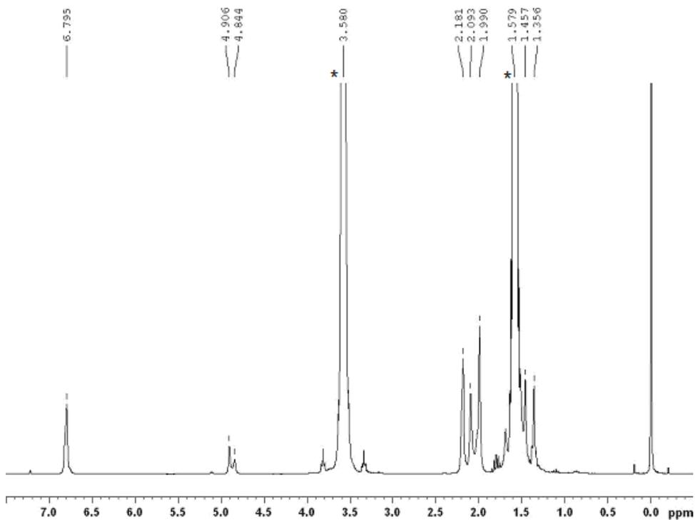
Figure 2.19 –  $^1\text{H}$  NMR spectrum of 2b in 1:1 THF: $\text{C}_6\text{D}_6$ . The THF solvent peaks are shown by the \* above them.
