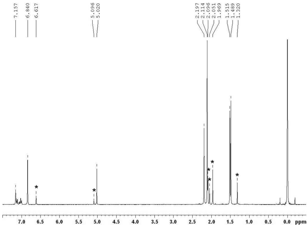
Figure 2.20 – The  $^1\text{H}$  NMR spectrum of 4b in  $\text{C}_6\text{D}_6$  at  $25^\circ\text{C}$ . The peaks with \* above them are uncoordinated ketoimine peaks. The crystals were shown to be pure material via the elemental analysis results in conjunction with the knowledge that only 0.4:1 molar ratio of toluene:4b remained at the time this NMR and the elemental analysis were performed.
