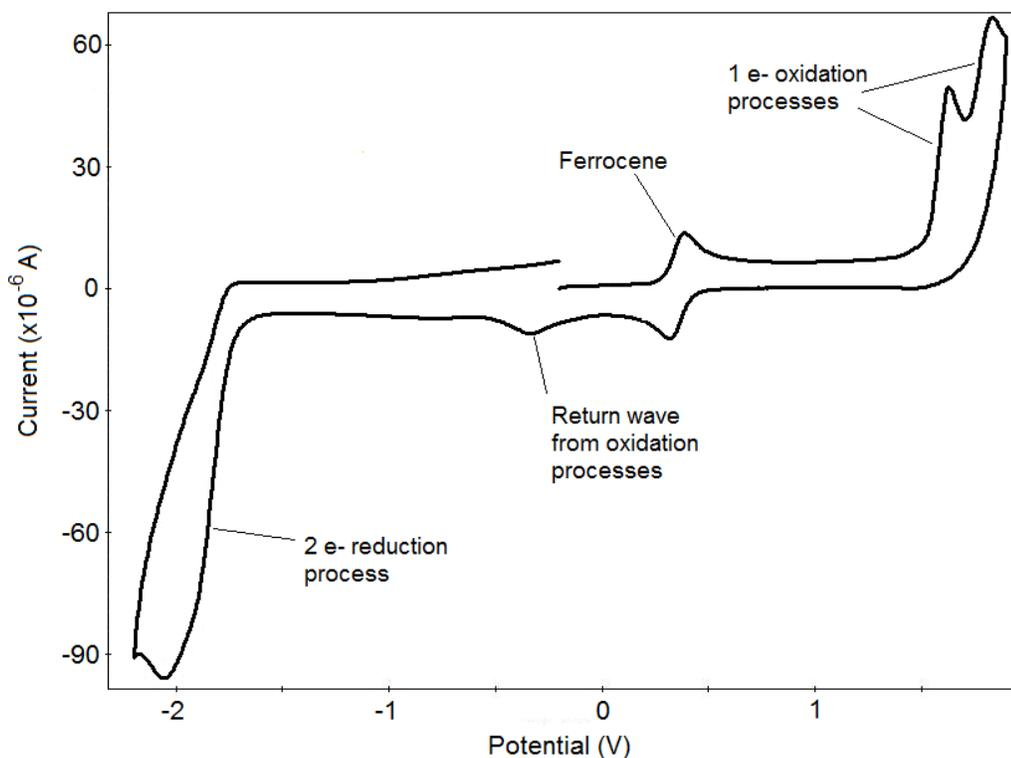
Figure 3.10 – CV of **5a** in  $\text{CH}_2\text{Cl}_2$  on a GC electrode at 0.7 M  $[\text{nBu}_4\text{N}][\text{PF}_6]$ ,  $\nu = 0.2 \text{ V s}^{-1}$  referenced to ferrocene at 0 V.
