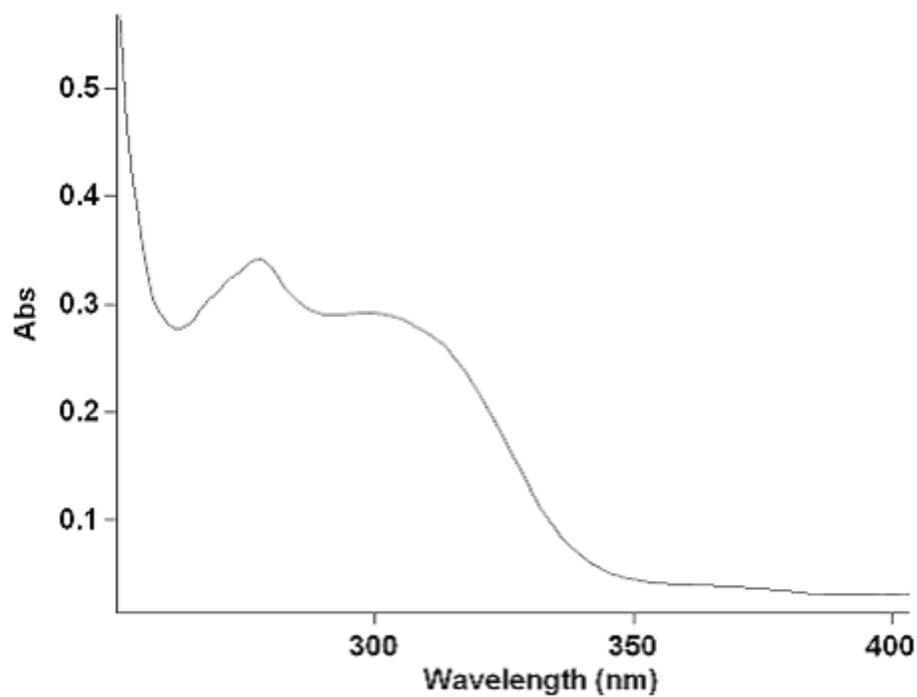
Figure 3.17 – UV/VIS spectrum for 5b in CH<sub>2</sub>Cl<sub>2</sub>. The calculated absorptions had too small of intensity to indicate on the above spectrum. The values are given in Table 3.5.
