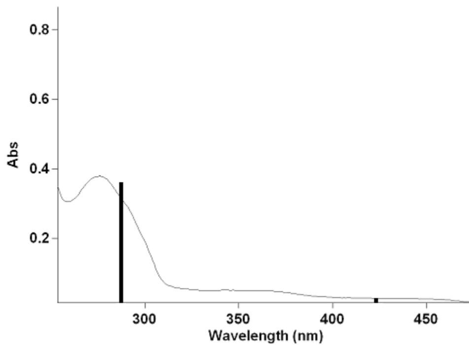
Figure 3.15 – UV/VIS spectrum of 7b (line) and calculated absorptions (bars) in CH<sub>2</sub>Cl<sub>2</sub>.
