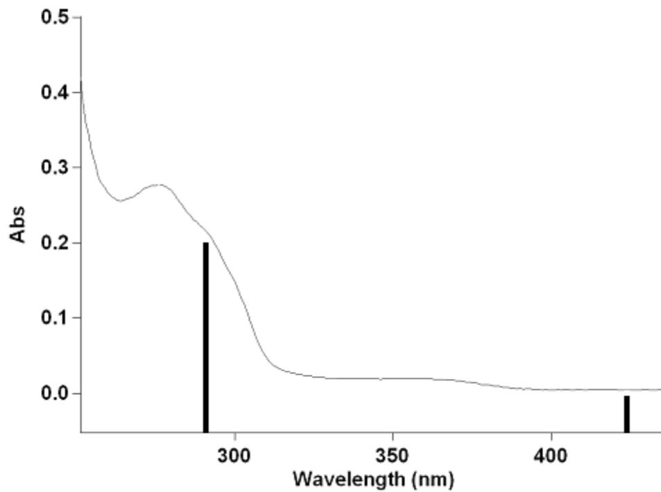
Figure 3.14 – UV/VIS spectrum of 6b (line) and calculated absorptions (bars) in CH<sub>2</sub>Cl<sub>2</sub>.
