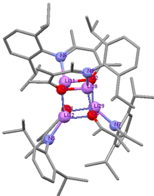
Figure 2.16 – B3LYP//6-31G(d) optimized structure of the  $S_4$  geometry for 4c (visualized with Mercury 2.2). The Li, N and O atoms are represented by spheres and the carbon atoms by tube-junctions. H atoms are omitted.
