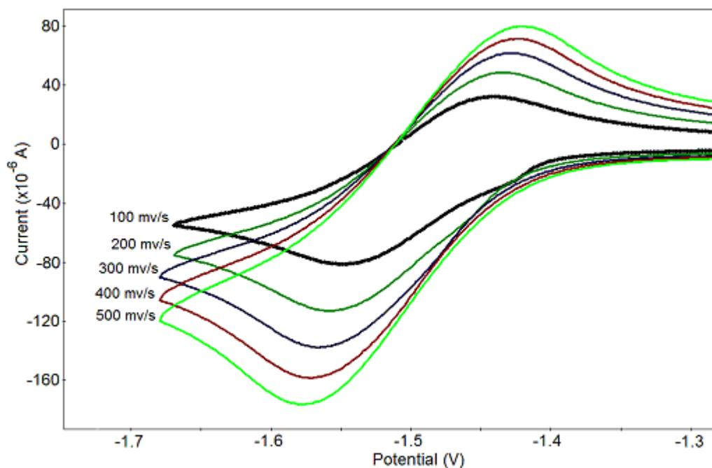
Figure 3.12 – CV of 4.65 mM 5b in CH<sub>2</sub>Cl<sub>2</sub> on a GC electrode at 24.5 °C, 0.7 M [tBu<sub>4</sub>N][PF<sub>6</sub>], at various rates referenced to ferrocene.
