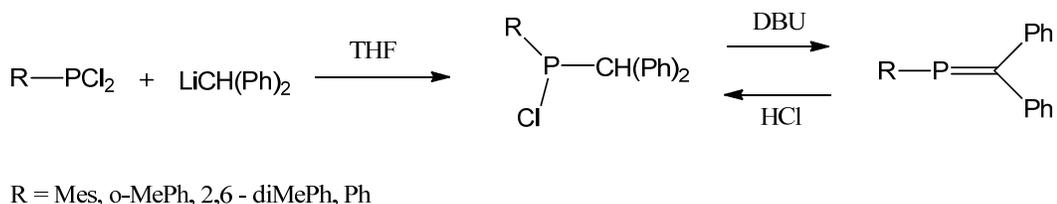
**Scheme 4.1 – The first reported 1,2-elimination reaction for the synthesis of phosphalkenes.**
