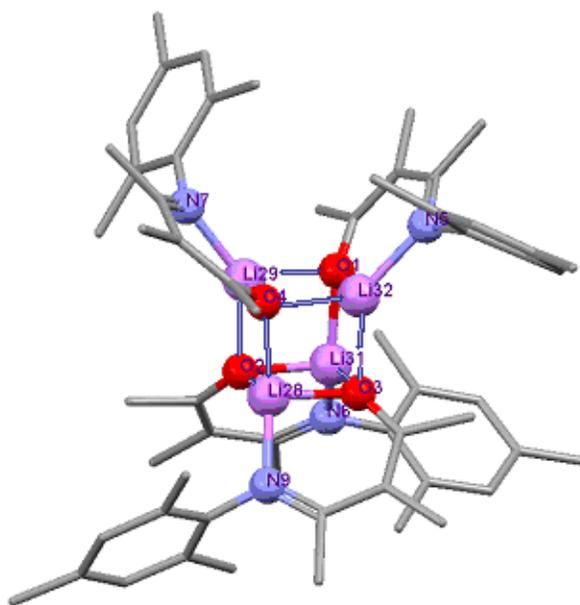
Figure 2.17 - B3LYP//6-31G(d) optimized structure of the  $S_4$  geometry for 4d (visualized with Mercury 2.2). The Li, N and O atoms are represented by spheres and the carbon atoms by tube-junctions. H atoms are omitted.
