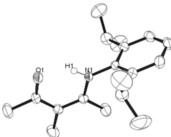
Figure 2.5 - ORTEP diagram of **1c** with all but the amine hydrogen atoms omitted for clarity (50% probability ellipsoids shown).
