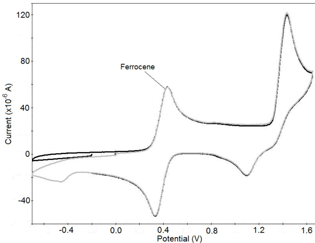
Figure 3.13 – CV of 4.30 mM 6b in  $\text{CH}_2\text{Cl}_2$  on a GC electrode at 24.5 °C, 0.7 M  $[\text{tBu}_4\text{N}][\text{PF}_6]$ ,  $\nu = 0.2 \text{ V s}^{-1}$  referenced to ferrocene. No reduction processes were observed, however the light grey line shows an additional return wave in the negative region after passing through the oxidation process first.
