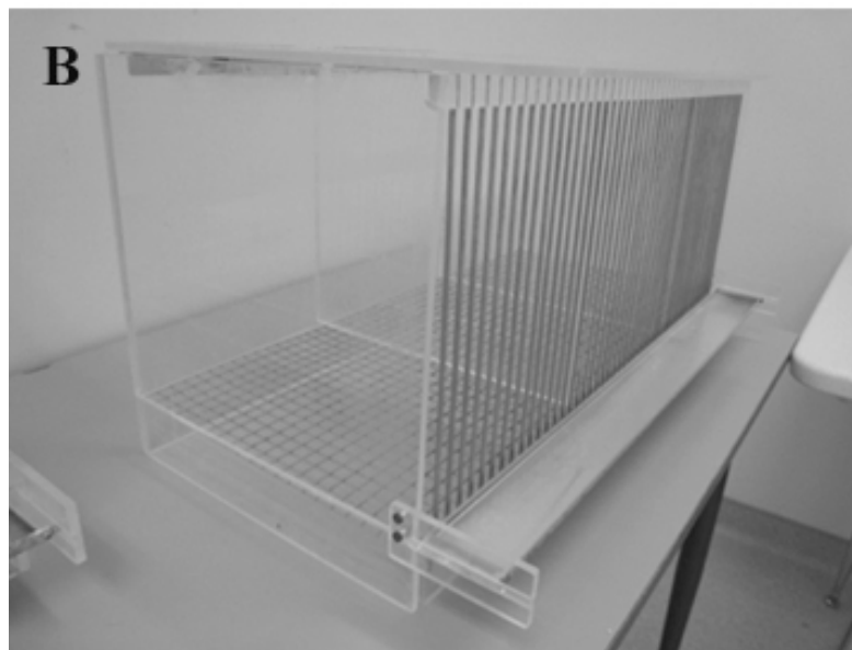
Figure 1.5. Tray-reaching apparatus. (A) front view of three attached tray-reaching boxes, (B) angular perspective of the apparatus for better view of the inside of the box as well as the food tray and metal grids floor.
