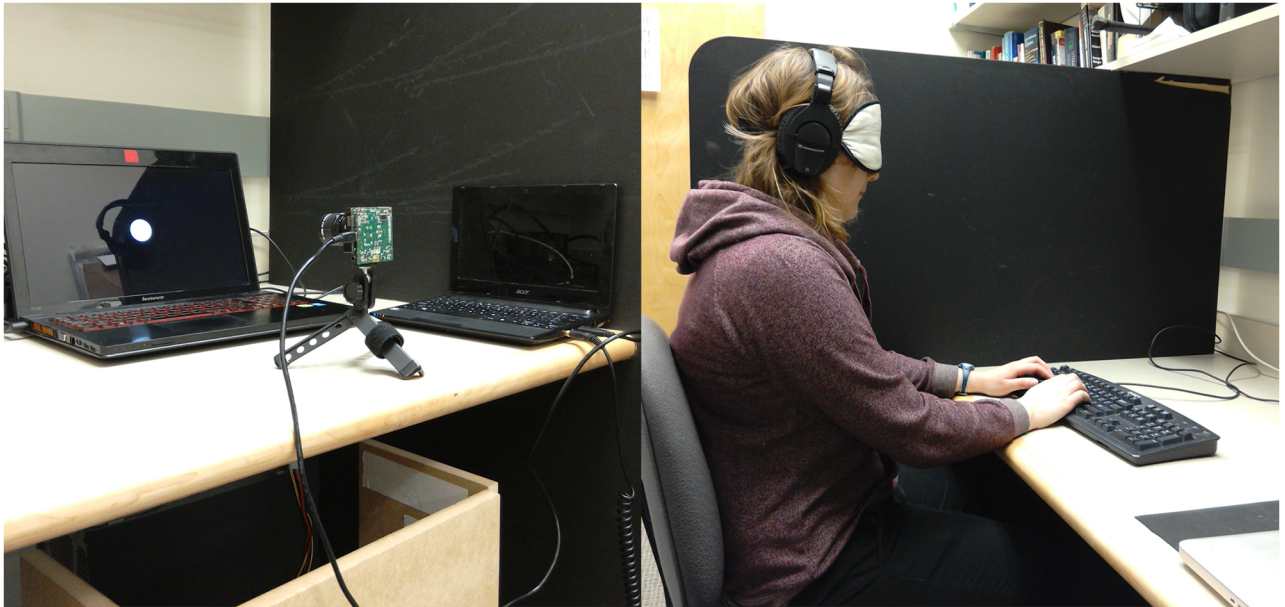
Fig 1. Experimental setup. Participants were blindfolded and positioned to the right of the black wooden separator to prevent any visual information from the laptop computer. The netbook was running the auditory augmented reality software and providing the headphone audio signal. The camera was positioned 42 cm away from the screen of the laptop to capture the entirety of the screen. The participant wore a blindfold to reduce the likelihood of visual distraction. The individual in this manuscript has given written informed consent (as outlined in PLOS consent form) to publish these case details.
