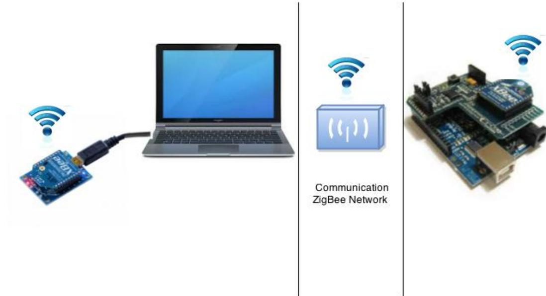
Figure 6.3: Simple communication between the sender and the receiver
