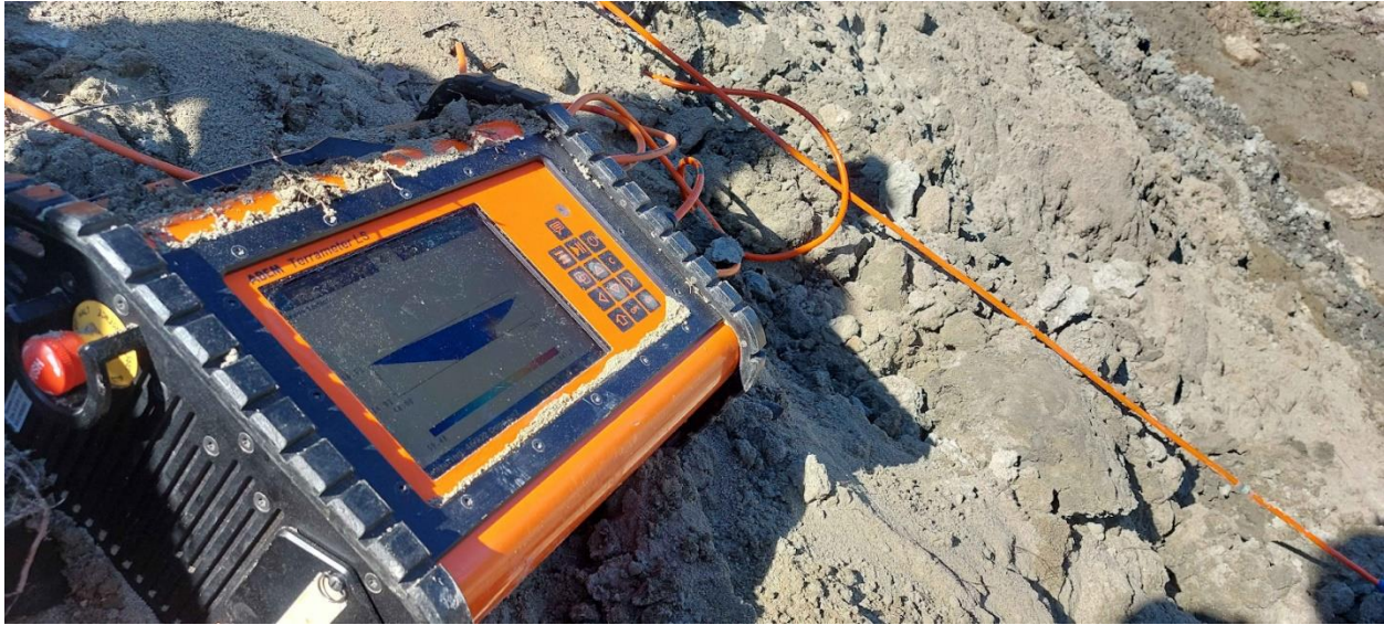
Fig. 2.12. An example of an ERT control unit in operation at the Takhini River Thaw Slump, YT. Photo taken June 2024.
