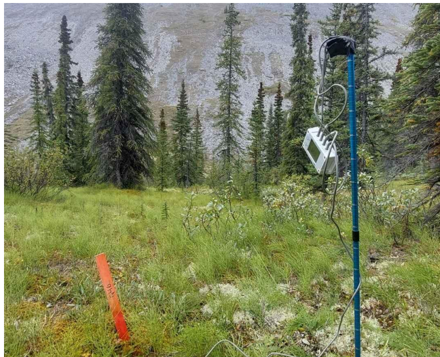
Fig. 2.10. A ground thermal profiling probe (right) made of an aluminium avalanche probe. Four thermistor wires are strung through the interior, with sensors placed at fixed intervals to record ground temperatures. Photo taken August 2023.
