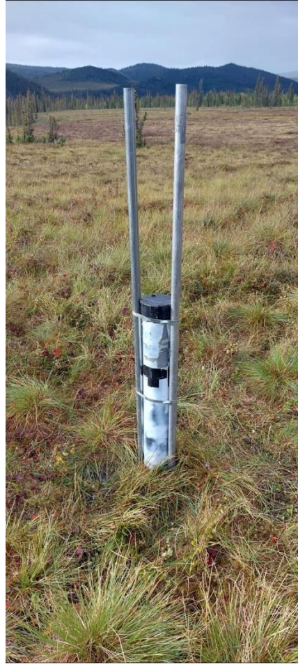
Fig. 2.11. An example of a permafrost borehole, located in Red Creek, Yukon. The borehole has been stabilised with metal piping. Photo taken August 2022.
