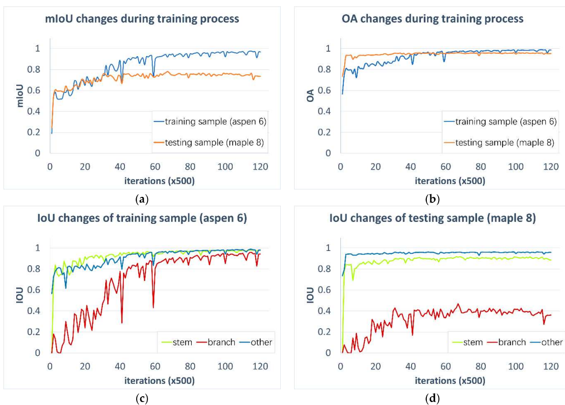
Figure 7. Relationship between accuracy changes and training iterations, for ‘aspen 6’ from training dataset and ‘maple 8’ from testing dataset: (a,b) fluctuation of mIoU and OA; (c,d) fluctuation of stem IoU, branch IoU, and other components’ IoU.
