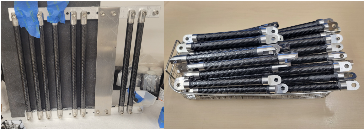
Figure 2.14: Assembly process of CFRP struts. Left: The assembly process using a jig to epoxy-bond eight CFRP struts at a time. Right: All fully assembled CFRP struts.
