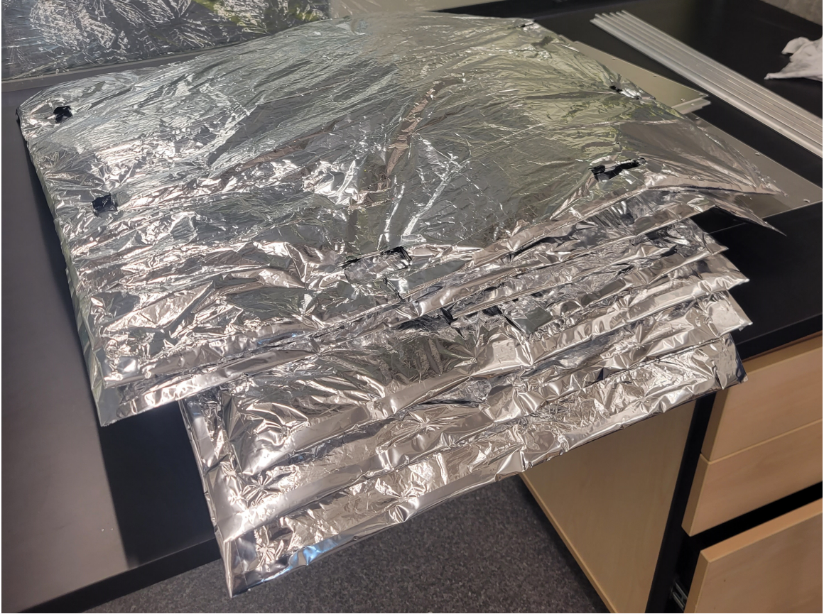
Figure 2.18: MLI blankets before they were installed onto the 45 K radiation shields.
