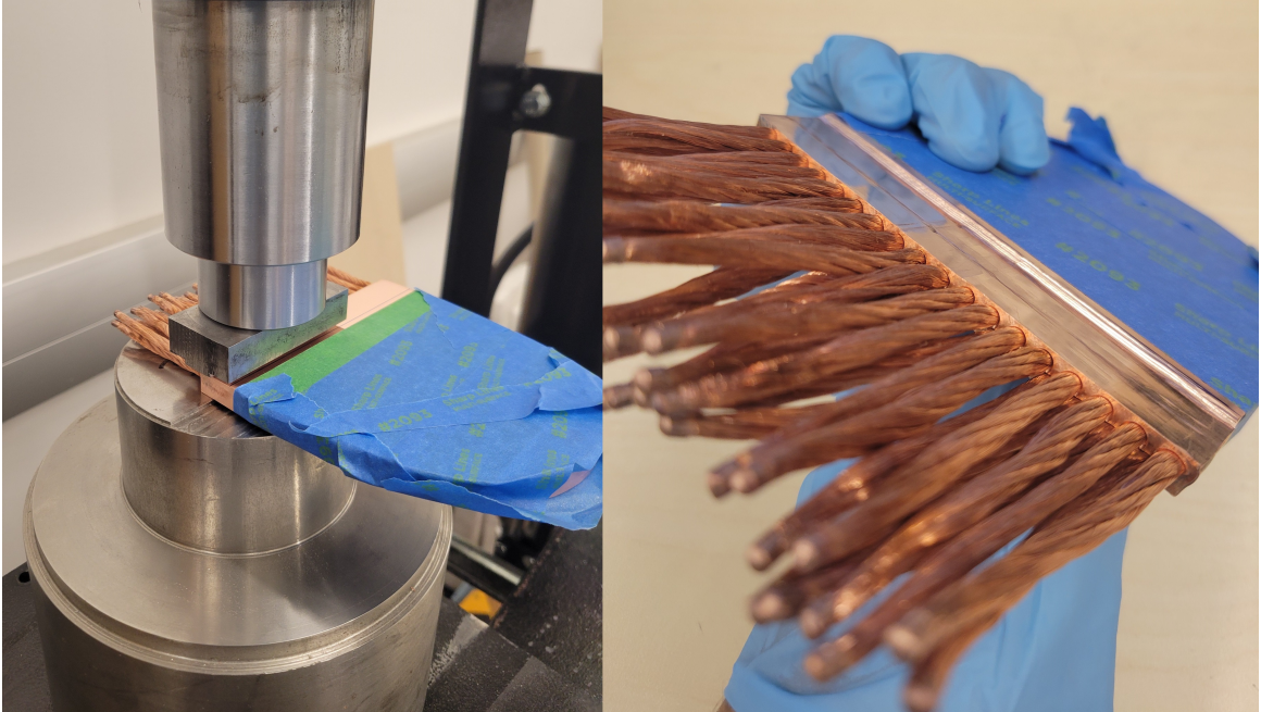
Figure 2.16: Process of manufacturing flexible thermal braids. Flexible copper cables are inserted into the ends of the braid plate. A hydraulic press is used to deform the braid plate and form a cold weld joint with the cables. Left: A hydraulic press is used to form the cold welds between a braid plate and flexible cables. Right: The results of the cold welding process on one end of the thermal braid.
