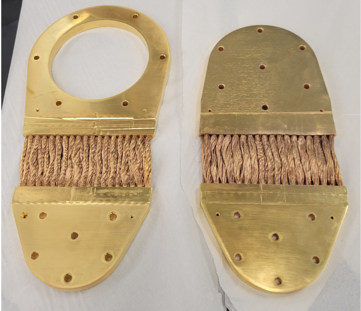
Figure 2.17: Flexible thermal braids after being pressed and gold plated. Left: 45 K braid. Right: 4 K braid.
