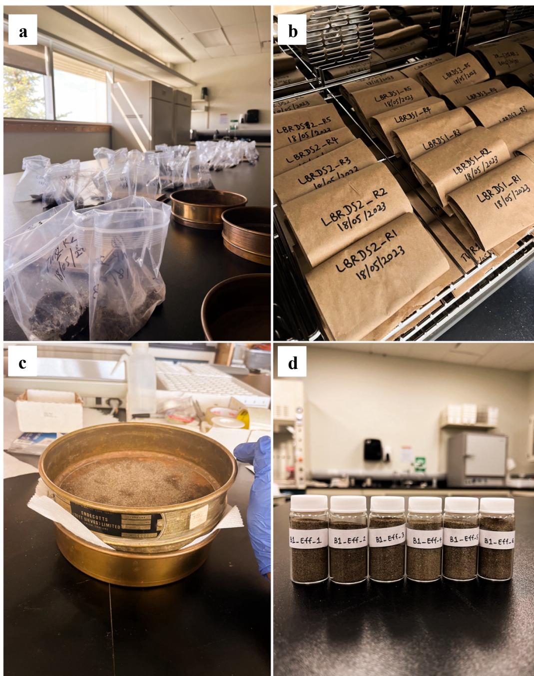
Figure 2.5: a) Sediment samples were collected from six replicates ( n = 6 ) at each sampling location. b) Upon return to the laboratory, the samples underwent air and oven-drying. c) Dried sediment samples were then sieved using a soil sieve with an 850 \mu\text{m} aperture. d) The samples were then transferred into 20 ml scintillation vials and sent for analysis of \delta^{15}\text{N} values using gas isotope ratio mass spectrometry at the University of Utah, USA.
