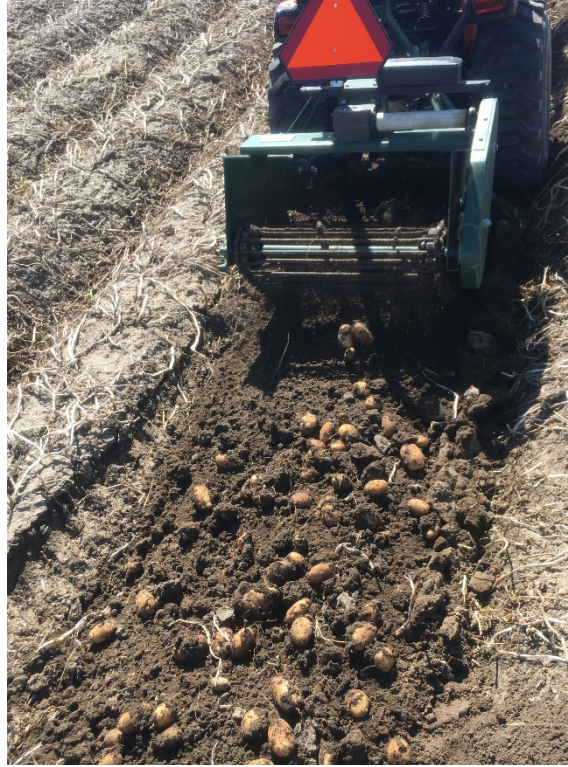
Figure 6 One row chain digger pulled by tractor. Used in all experimental fields, featured here in field NE 8. (photo by Colby Robertson)
