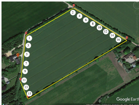
Figure 4.1: Layout of the 8-track benchmark field with on-field depot and working tracks.
