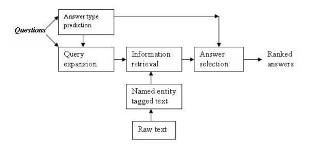
Figure 1.1: Common architecture of QA system
