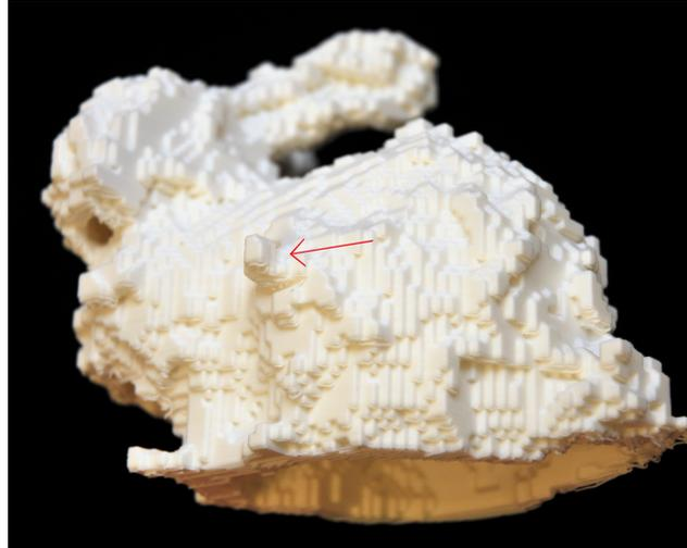
Figure 4.13: A protrusion on a scanned model.
