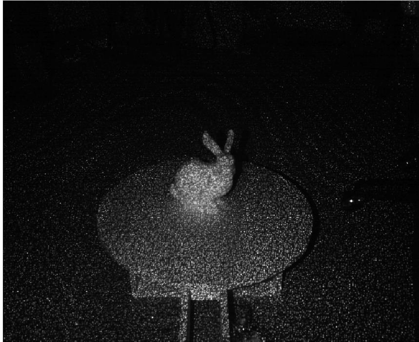
Figure 2.5: Infrared depth image taken from a Microsoft Kinect.
