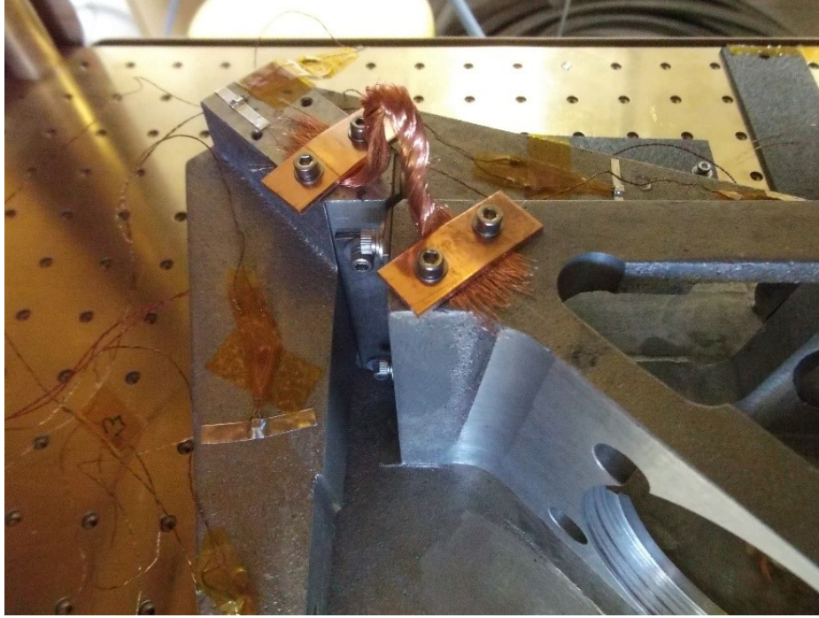
Figure 5.13: Flexible copper braid attached to pivot of the wishbone arm to aid cooling the arm.
