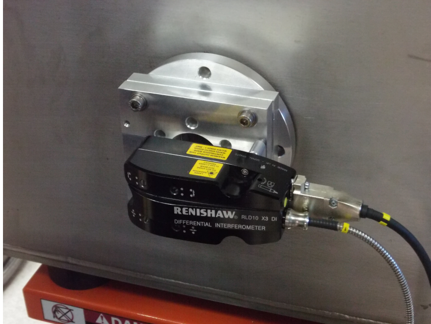
Figure 3.14: An image of the Renishaw RLD10 differential interferometer, mounted to the TFC with a custom-made set of aluminum plates. The plates allow for slight positional corrections to be made outside the cryostat, as well as easy detachment and re-attachment of the interferometer without realignment.
