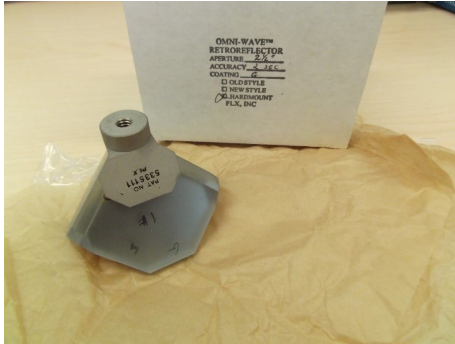
Figure 5.11: Replacement corner cube retroreflectors with Invar frame. These corner cubes were tested at 4 K and maintained alignment both while cold and on return to room temperature.
