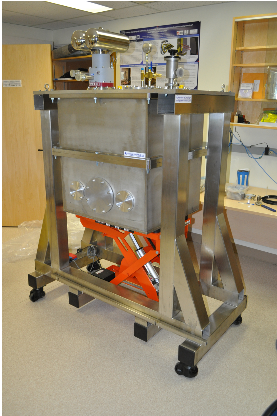
Figure 3.6: The Test Facility Cryostat after delivery to the University of Lethbridge. A single PTC, vacuum port, and liquid nitrogen inlet/outlet can be seen mounted to the upper plate. The horizontal split in the vacuum chamber allows for the bottom half of the chamber to be lowered by the scissor jack. Three blank flanges for the side apertures are also shown.
