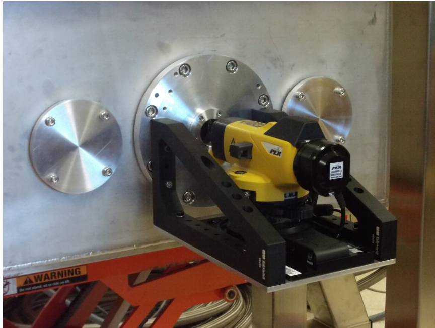
Figure 3.15: An image of the PLX electronic autocollimator mounted on one of the large viewports in the TFC. A shelf was constructed to hang from the viewport so that the autocollimator could be mechanically coupled to the TFC to reduced vibrational errors in the measurements. The viewport flange, shelf, and autocollimator can be removed from the TFC as a single unit.
