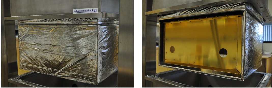
Figure 3.7: Removable radiation shield panels for accessing the 4 K volume.
