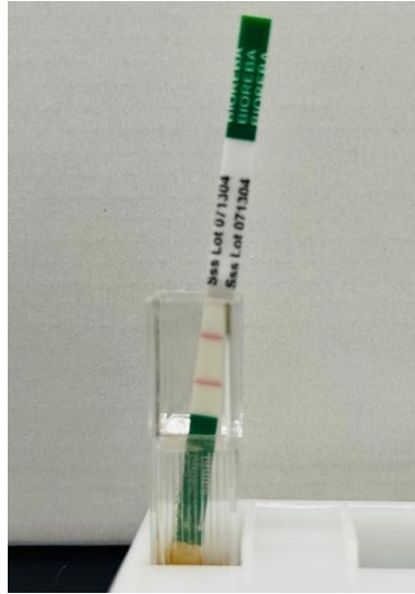
Figure A3.2: An Sss AgriStrip showing two visible bands: the upper band is the control line, confirming the test functioned correctly, and the lower band is the test line, indicating a positive result for the presence of S. subterranea DNA in the sample.
