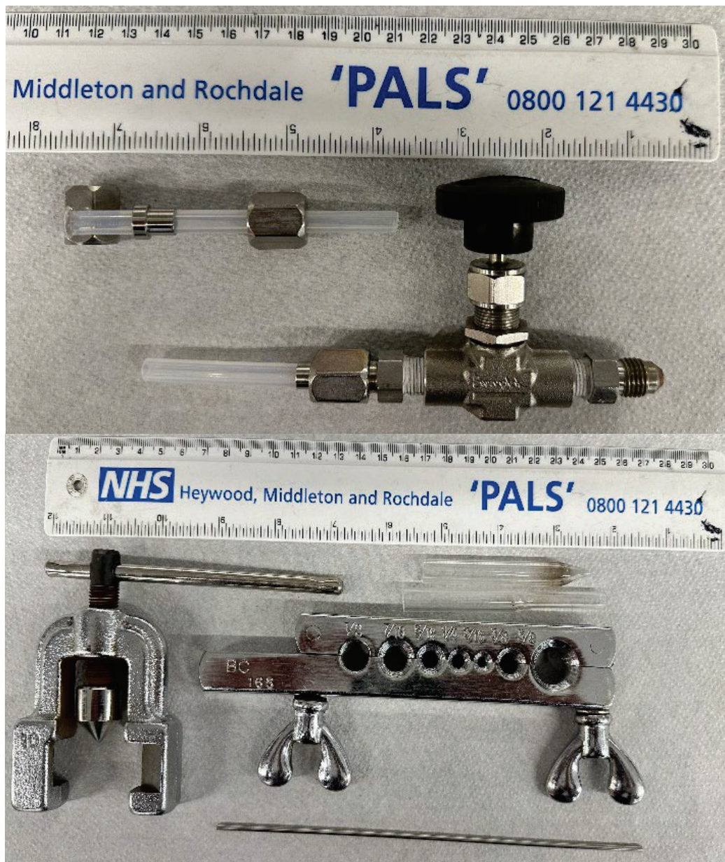
Figure 2.1. A 316-stainless steel (Swagelok SS-1KF2) valve with a flared ¼”-o.d. FEP tube with nut and sleeve (top) and equipment used to fuse thick-walled ¼” to 4-mm FEP and create the flare (bottom).
