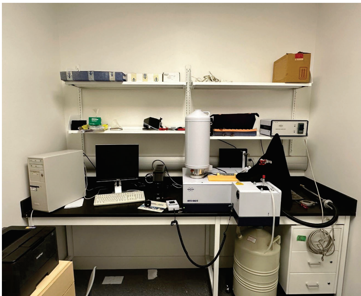
Figure 2.7. Bruker RFS-100 Raman spectrometer outfitted with a quartz beam splitter and liquid-N 2 cooled germanium detector.
