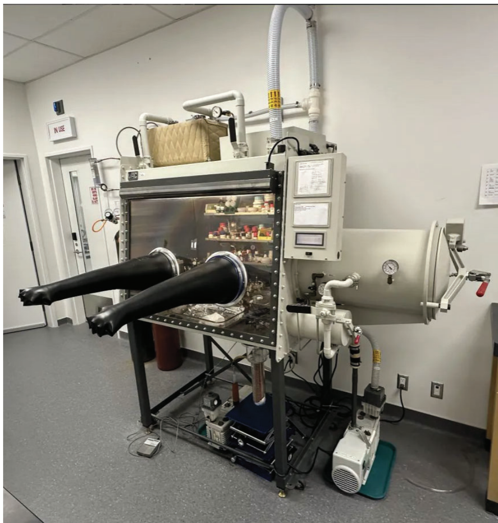
Figure 2.5. OmniLab, Vacuum Atmospheres dry box filled with a N_2 atmosphere and equipped with cold well filled with Cu BBs.
