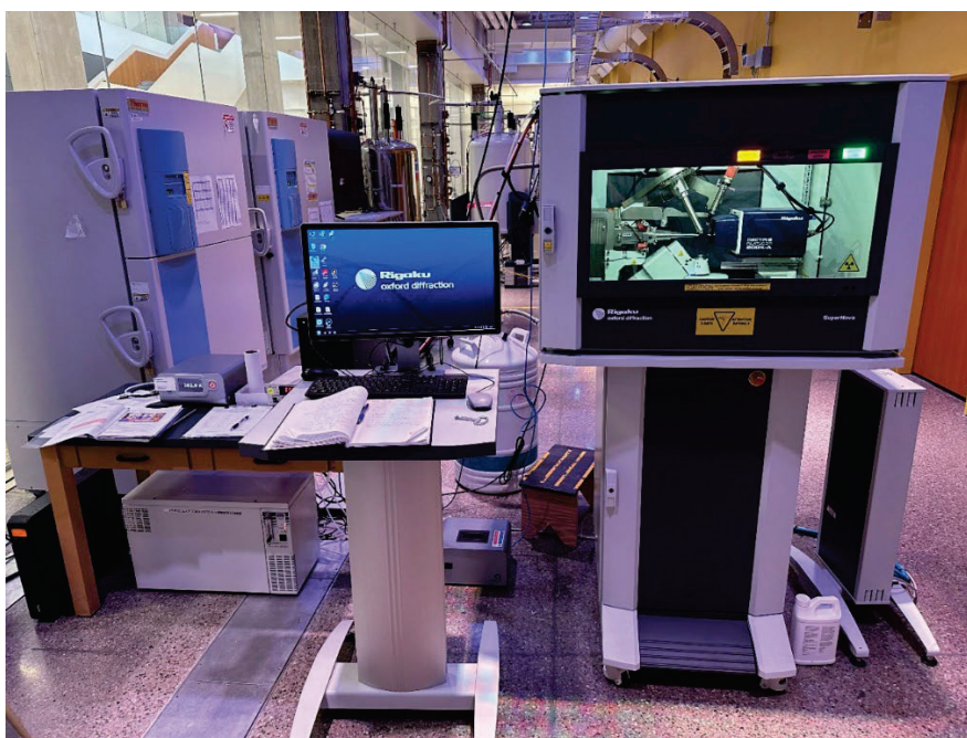
Figure 2.9. Rigaku SuperNova diffractometer equipped with a Dectris Pilatus 3R 200K-A hybrid-pixel-array detector, a four-circle \kappa goniometer, an Oxford Cryostream 800, and sealed MoK \alpha and CuK \alpha X-ray sources.
