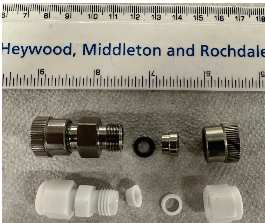
Figure 2.3. Ultra-Torr vacuum fittings (Swagelok) (top) PTFE vacuum fittings (Swagelok) (bottom) partially disassembled.
