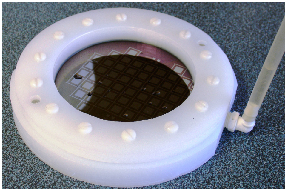
Figure 3.34: The Teflon ® etch boat loaded with a wafer.
