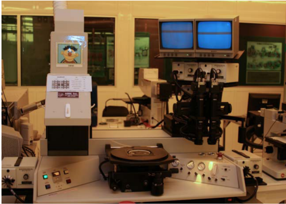
Figure 3.15: ABM infrared mask aligner.
