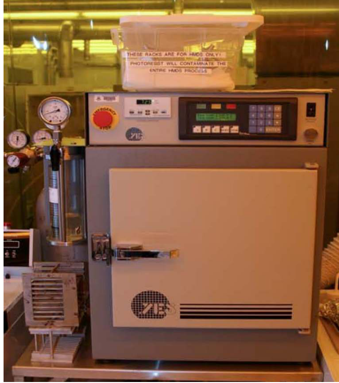
Figure 3.12: The vacuum bake/vapor prime (HMDS) oven.
