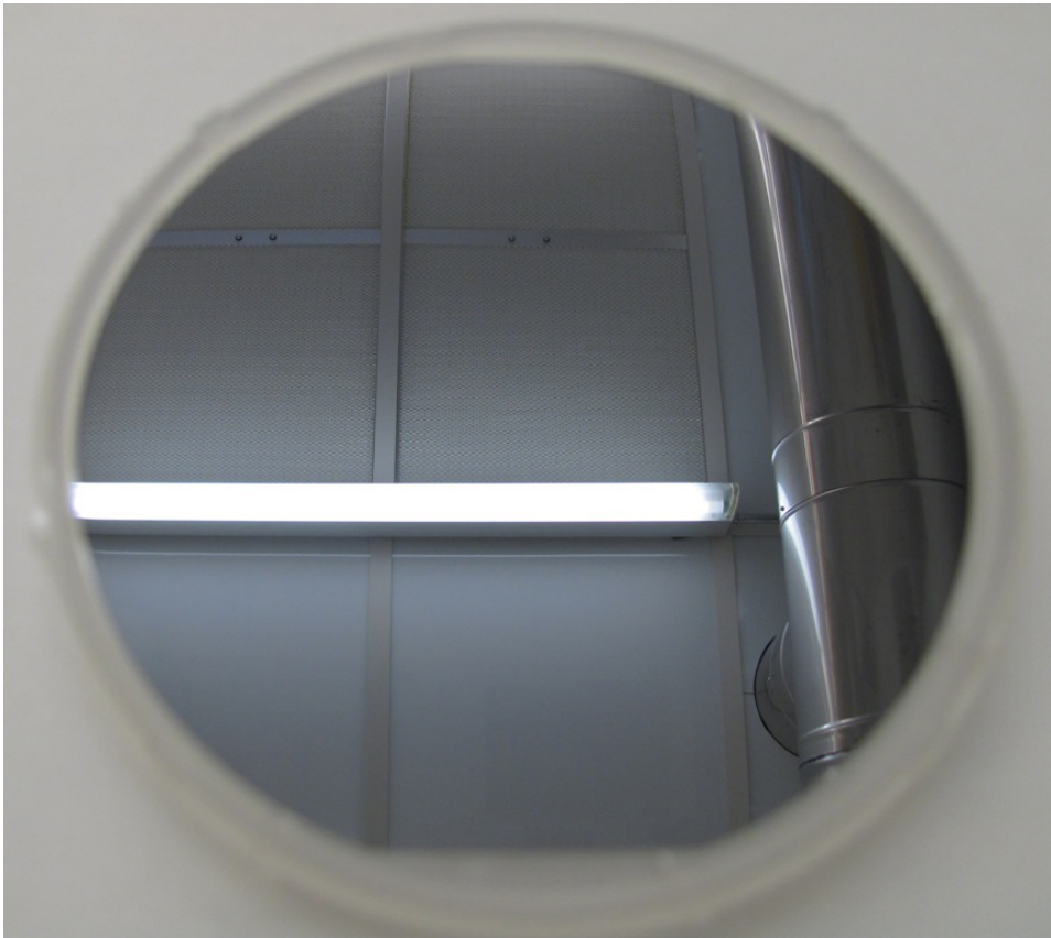
Figure 3.18: A Si wafer deposited with a layer of Nb film.
