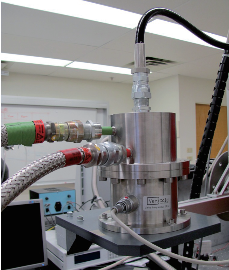
Figure 5.8: High-pressure and low-pressure flexlines connected to the rotary valve of the pulse tube cooler.
