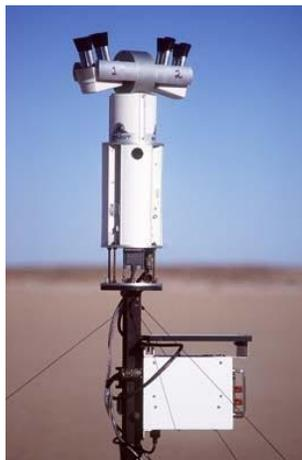
Figure 2.2 : The PARABOLA-3 dual-axis, up and down looking, three-band radiometer, downloaded from <http://www-misr.jpl.nasa.gov/mission/vinstrum.html>, 20 May, 2010.
