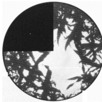
Figure 3.5 : Fisheye photo as viewed by the LAI-2000 fixed with a 270° lens attachment (Licor, 2010). The 270° lens attachment allows light to enter the lens at 270° and blocks light into the remaining 90° (dark region). Figure taken from Licor (2010), and does not correspond to any crop type, DAP or wavelength related to this study.
