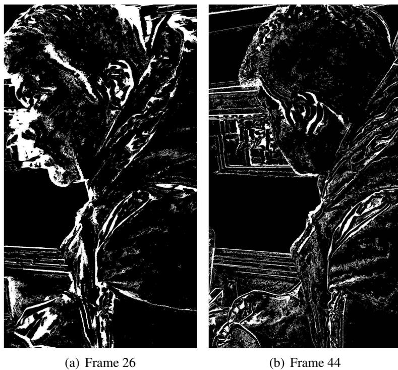
Figure 3.13: DVS events corresponding to the example frames in Figure 3.12. Pixels with DVS events are shown in white.
