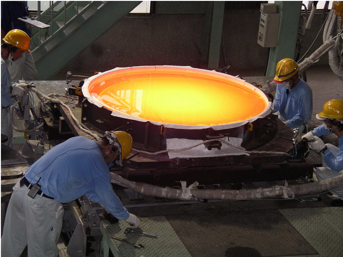
Figure 2.1: One mirror segment being poured for TMT (Photo Credit: Thirty-Meter Telescope Project)
