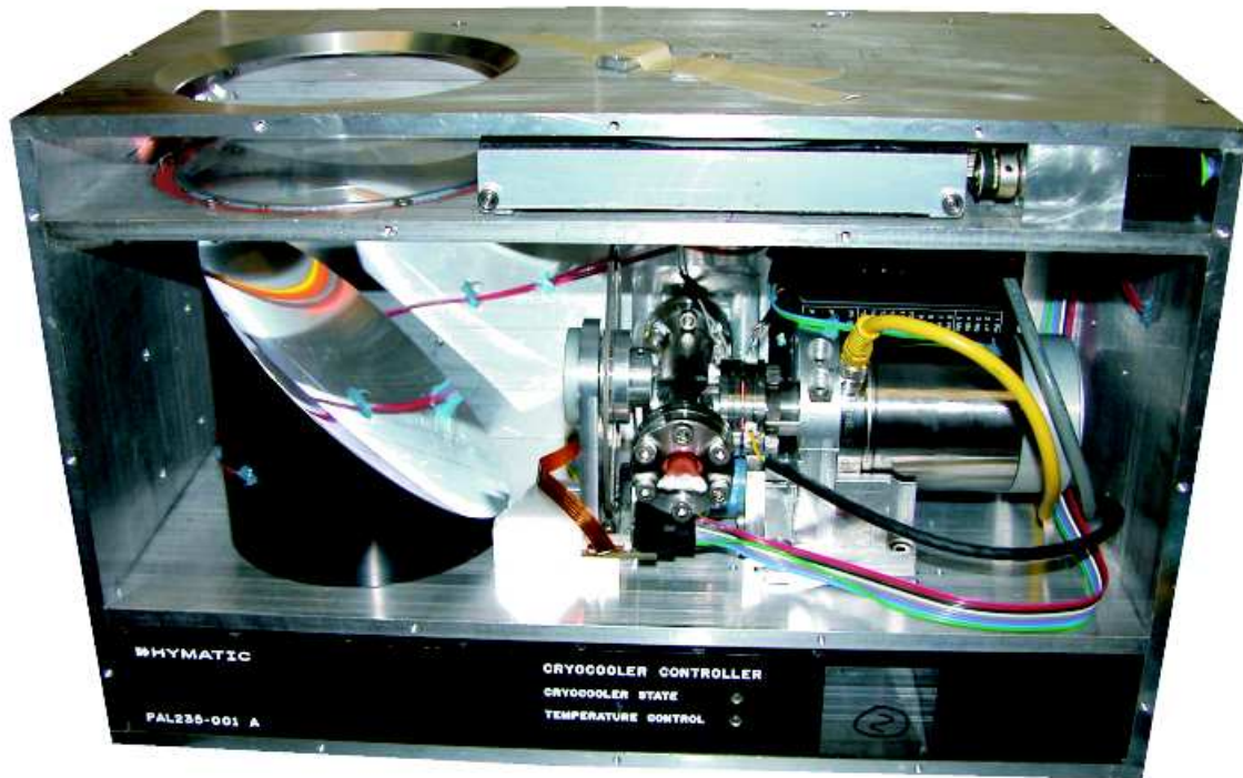
Figure 1.6: Photo of the optical side of the IRMA instrument. The shutter/internal blackbody is open. Components including the detector assembly, the cooler controller, chopper wheel, and paraboloid mirror can be seen from this side of the unit. The far side (not pictured) houses the electronics.
