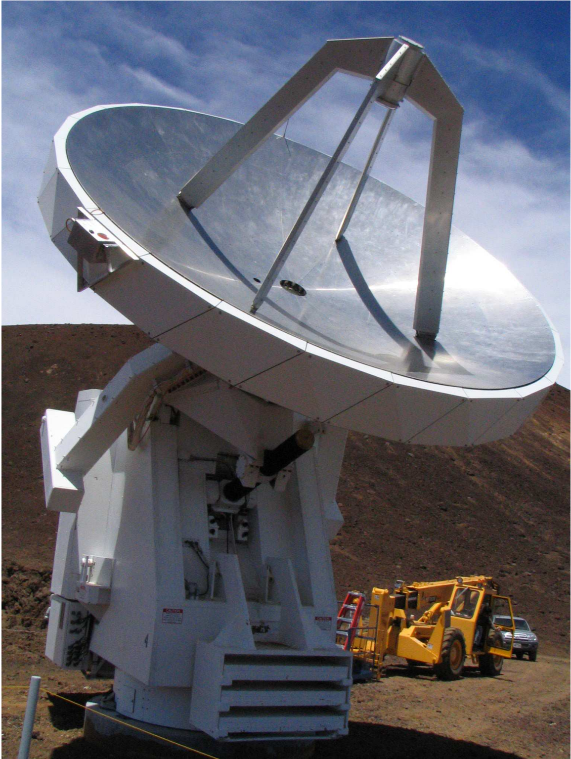
Figure 1.7: An IRMA unit affixed to the primary reflector (left edge) of this radio telescope in the Smithsonian Millimeter Array (SMA) in Hawaii.
