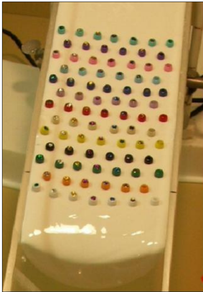
Fig 3.6 – Detail of the 85 points included on the strain grid prior to flow. Strain grid is 13.5 cm wide and 24.0 cm long with a total area of 324 cm 2 before flow begins.
