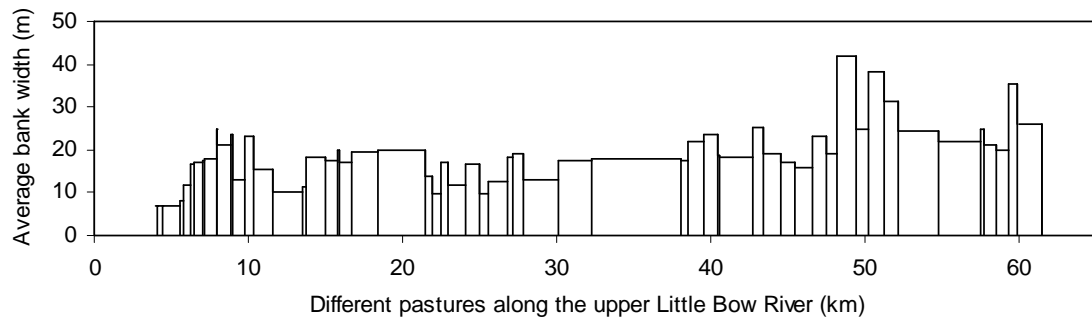
Figure 2-11 Average channel width calculated for different fenced parcels of land along the upper Little Bow River.
