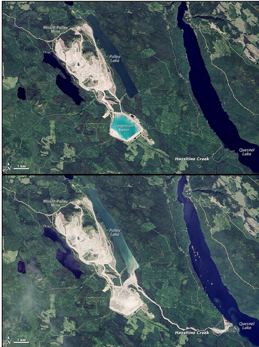
Figure 1. 1 Satellite images before (top) and after (bottom) the Mount Polley Mining Corporation tailings impoundment breach of August 4, 2014 (images from Google (n.d.)).
