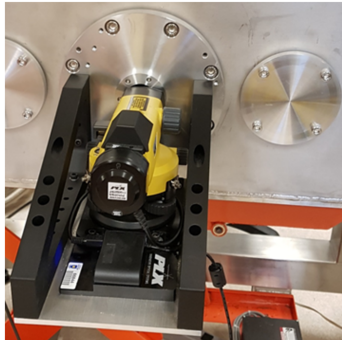
(b) Autocollimator setup on the test facility cryostat.
