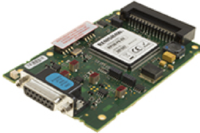
Figure 5.2: The RPI20 parallel interface card is connected to the RLE10 laser encoder through the 15 pin din connector located on the front of the card. The rear of the card has a Japanese Aviation Electronics (JAE) 60 pin connector which needs to be connected through the designed shield to the ARTY FPGA.
