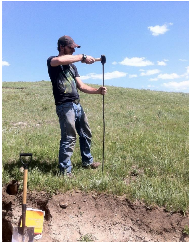
Figure 3.3: Photograph showing the knocking pole and hammer in use [summer 2018].
