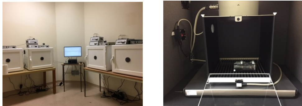
Figure 4. pre-pulse inhibition experiment. (Left) the PANLAB Harvard Apparatus consists of four acoustic startle boxes connected to the computer hard drive. (Right) shown the set up inside the acoustic startle box.
