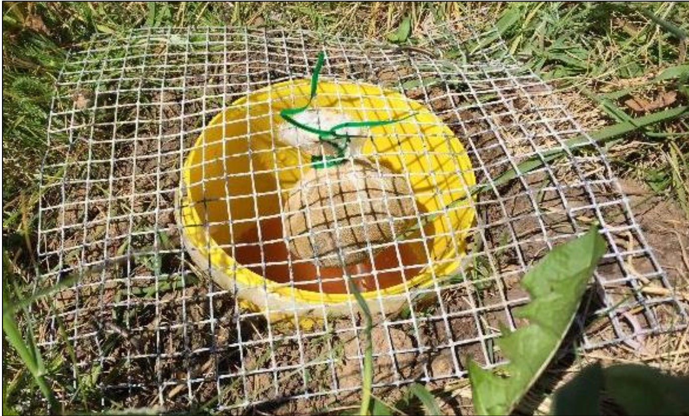
Figure 3.3. Design of pitfall trap used in the current study. A metal grid over the mouth of a 2 L pail supports a bait of cow dung wrapped in cheese cloth, and excludes small animals. Non-toxic antifreeze in the pail is used as a preservative.
