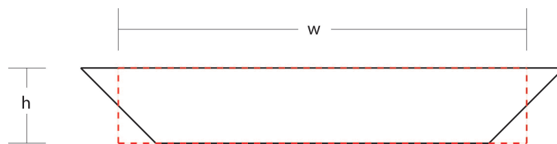
Figure 6.2: Cross-sectional schematic of cantilever. The cantilevers are manufactured such that they are slightly wider at the top where the detection laser is reflected off as compared to the sample side. This causes an increase of up to 30% of the reflecting surface, increasing the amount of the incident beam that is reflected toward the detector.
