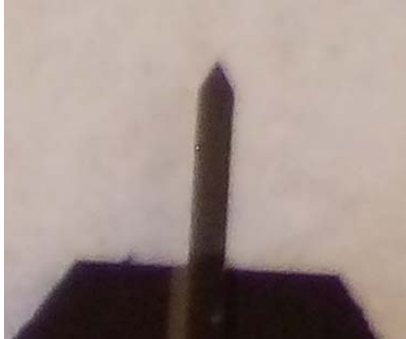
Figure 6.3: Zoomed in photograph of the 500 \mu\text{m} cantilever. This image shows the pointed tip which causes the last 10% of the tip to deviate from the expected rectangular shape.
