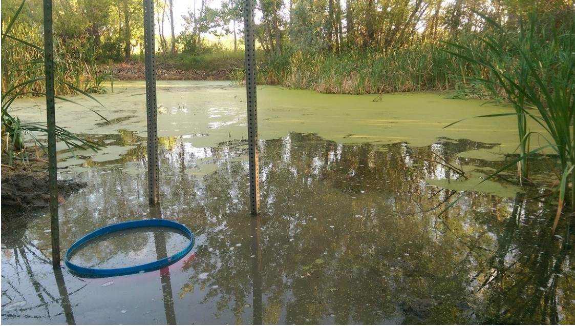
Figure 5-5. FLOA submerged after increase in water level. The mesh-barrier on the FLOA became inundated with mud after contacting the bottom, weighing down the apparatus.
