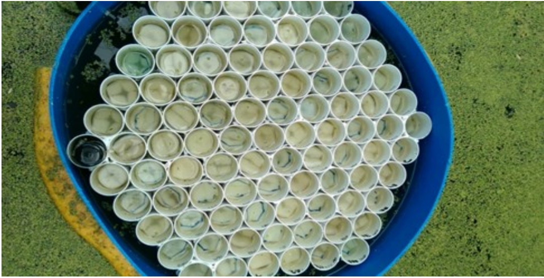
Figure 5-3. FLOA with additional foam in observational cells. The foam was added to prevent random fronds from emerging into the observational cells.
