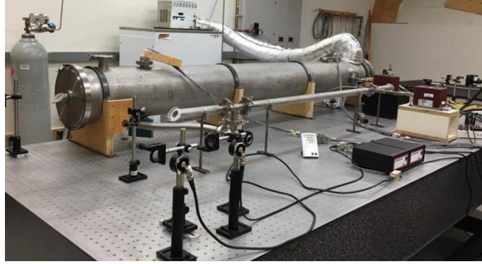
Figure 3.2. A recent photo of the tunable diode laser spectrometer located in our lab.
