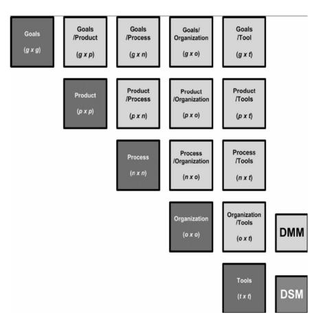
Figure 2.18: DSM and DMM modeling framework [9]
