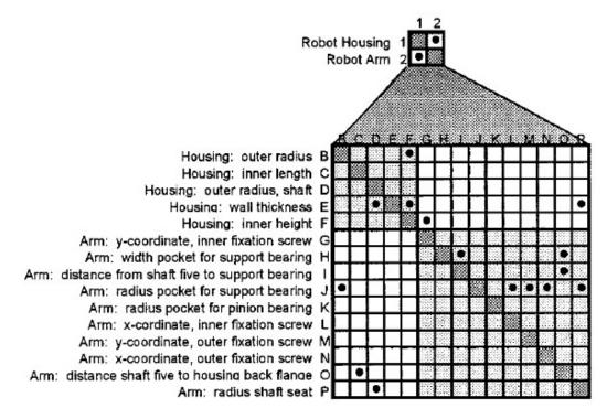
Figure 2.11: Parameter-based original DSM of robot arm design [25]
