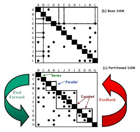
Figure 2.14: DSM after partitioning [30]
