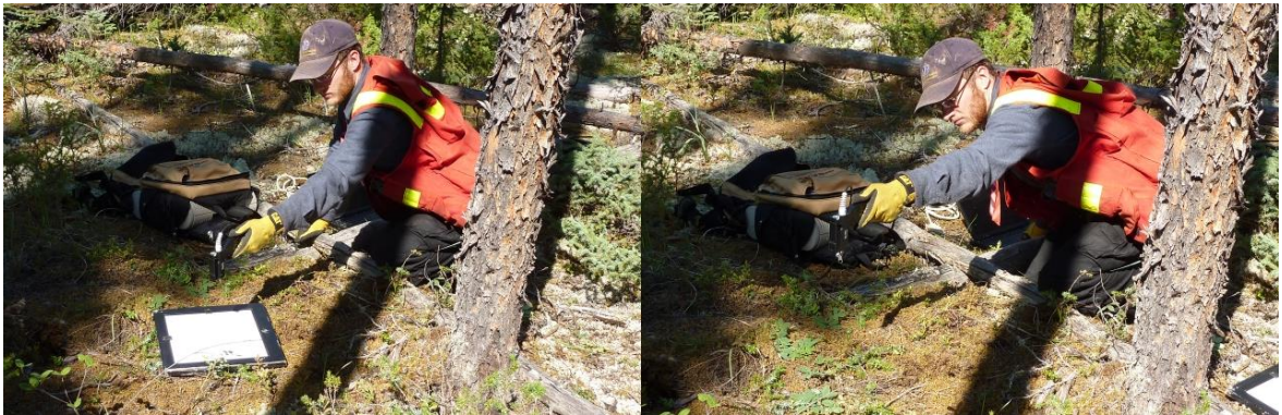
Figure 11: White reference measurement (left) and target measurement (right).
