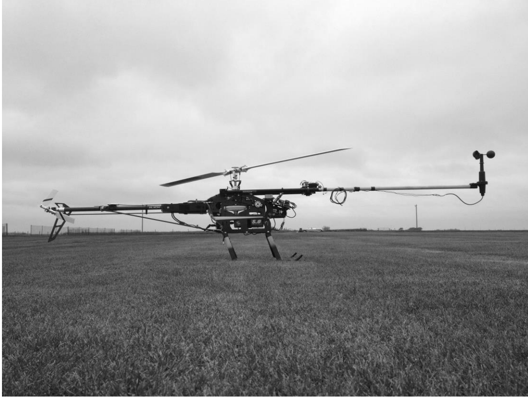
Figure 2.1. Profile view of the sUAS. The boom with anemometer is mounted forward of the flying surfaces to minimize wake turbulence. The collection payload is located just forward of main mast as close as possible to center of gravity to maintain positive flying characteristics.
