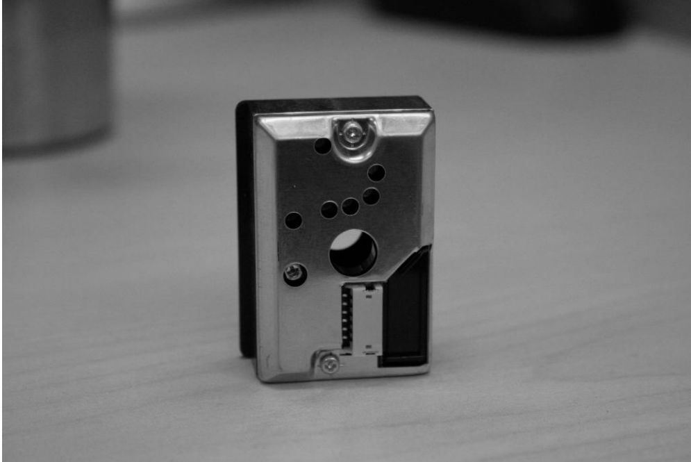
Figure 3.1. An image of the Sharp GP2Y1010 sensor showing the sensor hole (centre of enclosure) and interface connection pins.
