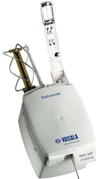
Figure 5.1: A Vaisala RS92-SGP radiosonde instrumentation package. The unit is approximately 220 \times 80 \times 75 mm, weighing typically 250 g. Image courtesy of Vaisala Inc.
