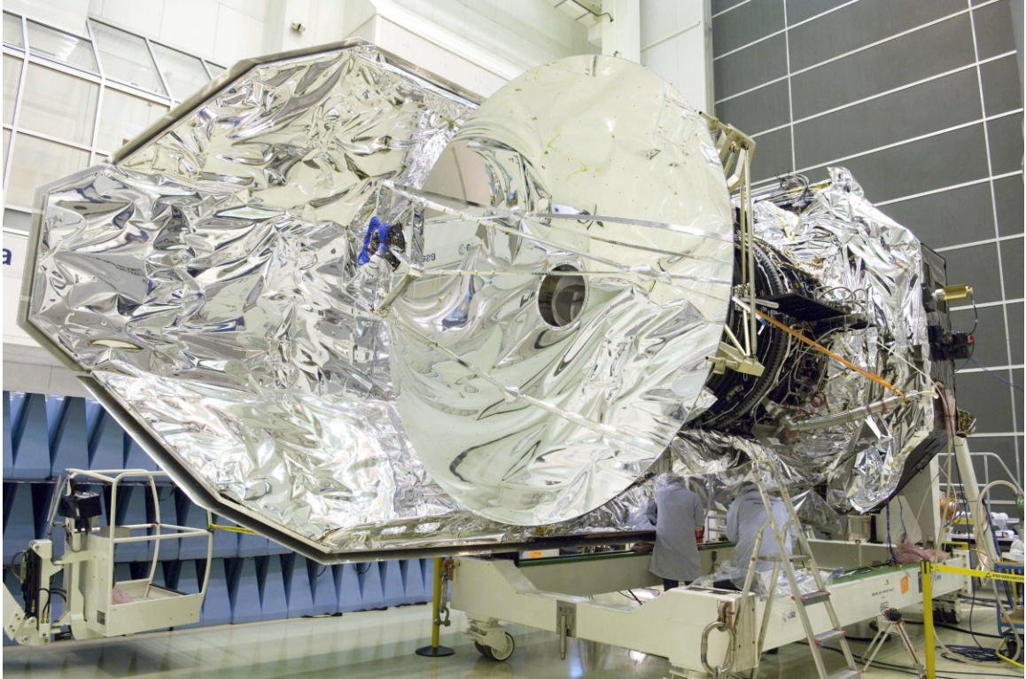
Figure 1.1: Photograph of the fully assembled Herschel Space Observatory. Photo: ESA
