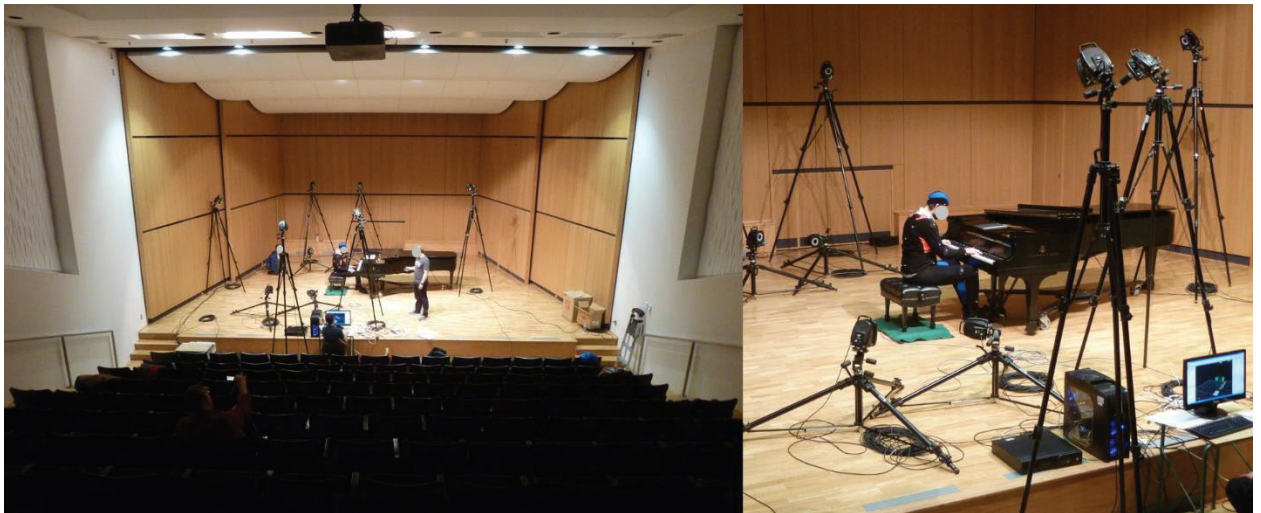
Figure 13: The experimental set-up of the motion capture system in the concert hall.
