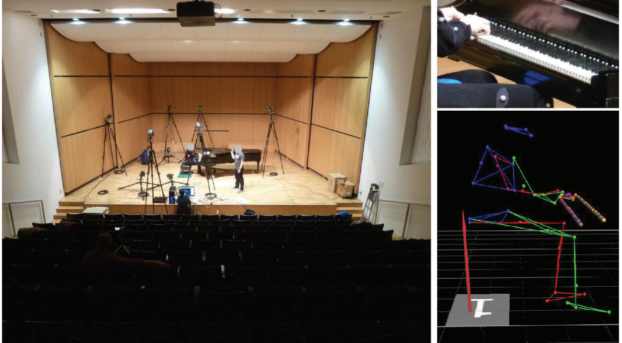
Figure 7: The Experimental Set-up (left), with Markers placed on the Participant and Keyboard (top right), and a Sample Frame from the Computer-generated Model (bottom right).
