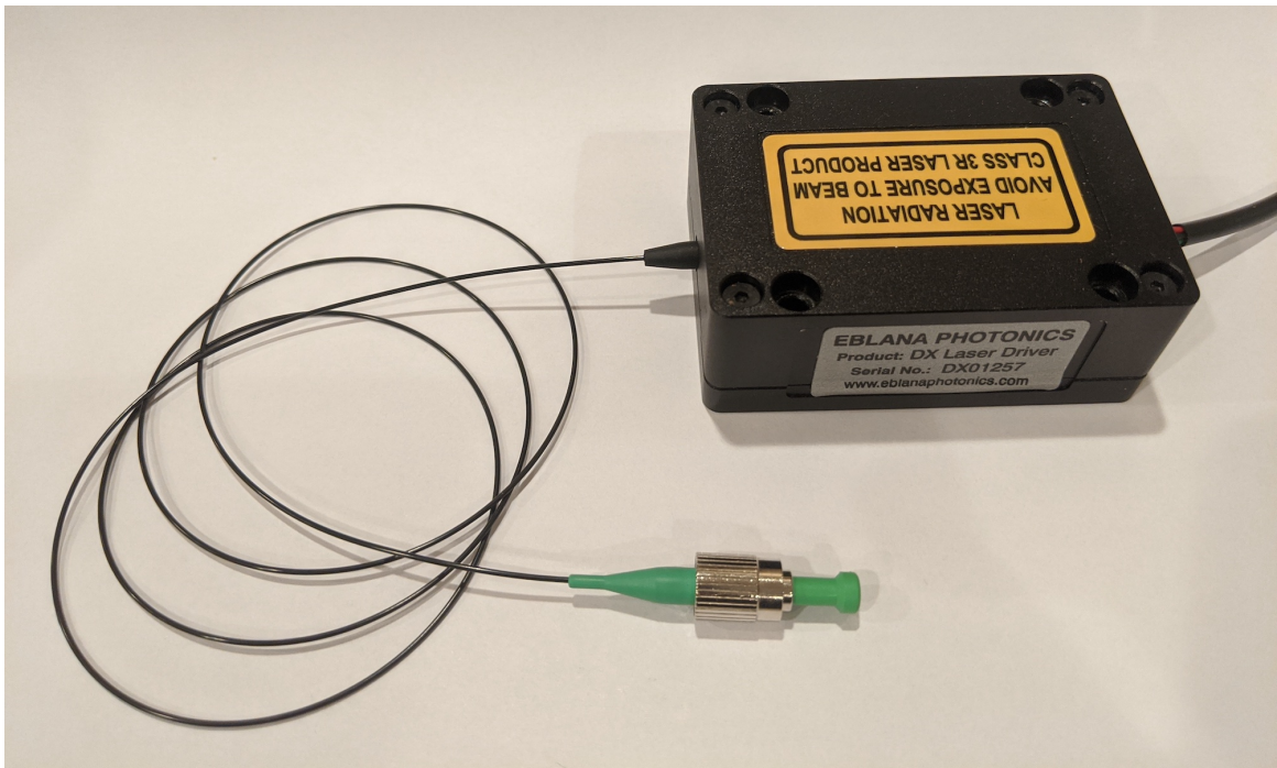
Figure A.1: An Eblana DX1-DM laser module. The laser output is coupled to an FC/APC terminated single-mode fibre.
