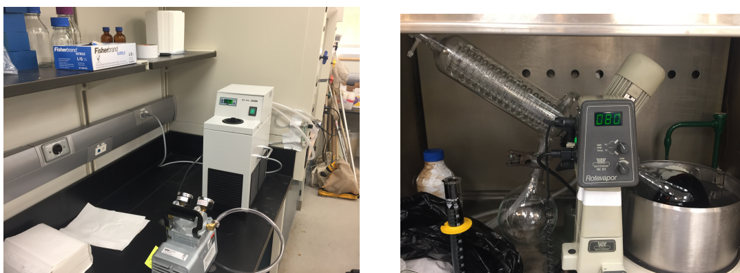
Figure A1 Lauda WK 300 circulation chiller and vacuum pump. Chiller set at 4°C and vacuum pump set to 13 L/min (left). Buchi-121 Rotary evaporator. Entering at the top of the condenser is an 8mm airline tube connected to a 9mm plastic pipet tube that extends to the beginning of the evaporation flask (right).
