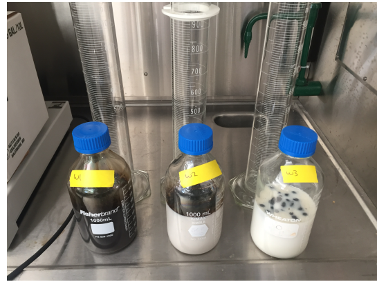
Figure A2 One-liter glass bottles filled with 30 mL weathered dilbit, 12 g kaolin and 600 mL freshwater. Prior to mixing (left) and after 16 h mixing on table shaker (right). For both pictures the left bottle is W1 (9.7% mass loss), the middle bottle is W2 (19.3% mass loss), and the right bottle is W3 (29.0% mass loss).
