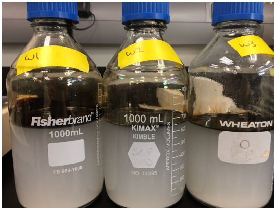
Figure A2 One-liter glass bottles filled with 30 mL weathered dilbit, 12 g kaolin and 600 mL freshwater. Prior to mixing (left) and after 16 h mixing on table shaker (right). For both pictures the left bottle is W1 (9.7% mass loss), the middle bottle is W2 (19.3% mass loss), and the right bottle is W3 (29.0% mass loss).
