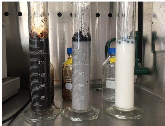
Figure A3 One-liter graduated cylinders filled with a mixture of 30 mL of dilbit weathered to varying degrees, 12 g kaolin and 600 mL freshwater that were mixed on a table shaker for 16 h. Immediately after addition to the cylinder (a) after 24 h settling (b). For both pictures, the left cylinder is W1 (9.7% mass loss), the middle cylinder is W2 (19.3% mass loss), and the right cylinder is W3 (29.0% mass loss).
