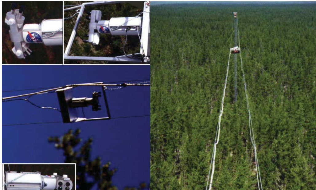
Figure 3.11: The PARABOLA-2 goniometer system mounted upon the tram above the canopy at the BOREAS SSA OJP site (NASA, 1994)
