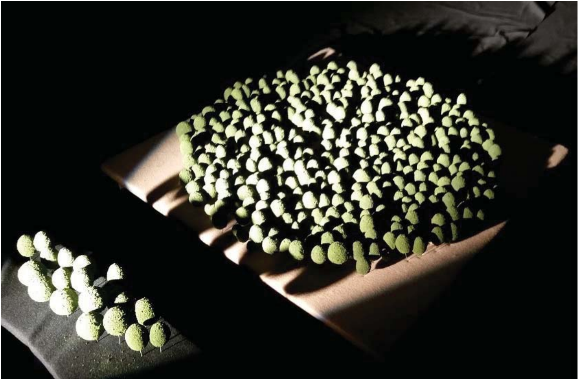
Figure 3.5: Fully constructed 60% crown closure physical model forest of spheroids-on-sticks viewed at an oblique angle.
